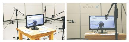
The noise of computer and servers tested by VoiceX is mainly measured according to the test method given by GB/T 18313 (which equivalent to the international standard ISO 7779). VoiceX is equipped with a low inherent noise semi-anechoic chamber and high-sensitivity microphones to measure sample's sound power level, sound pressure level at the operator's position and the bystander's position accurately.
