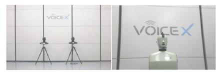
Sound quality parameters mainly include loudness, sharpness and roughness. VoiceX has library with all kinds of sound quality parameters analysis, such as FFT analyzer, CPB analyzer (1/n octave), the prominent discrete tone analyzer, loudness/ sharpness/ modulation analyzer and so on, which can meet all kinds of test requirements.
