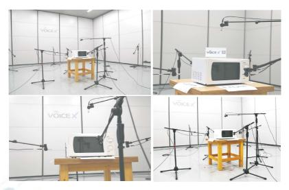
According to IEC 60704, GB/T 4214 and other series standards, VoiceX laboratory can hold household appliances test, such as air purifier, humidifier, microwave oven, etc. Test parameters include sound pressure level, sound power level, and sound quality parameters.
