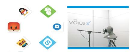
Nowadays, as the communication technology of VOIP becomes more and more mature, social APP communication is becoming more extensive. The VoiceX lab is equipped with a large anechoic chamber and professional head (Type3.3). The reference computer is equipped with a special UCX sound card to ensure the quality and accuracy of audio transmission. We also can customize special test project to meet your needs.
