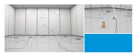
VoiceX laboratory has professional sound power testing equipment, which can config the microphone with hemispheric envelope or rectangular envelope, measure the sound power level of noise source, according to ISO 3744, ISO 3745, GB/T 3767 and other series of standards.
